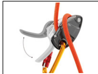
Anti-panic handle: if the user pulls too hard on the handle, the anti-panic function brakes and stops the descent automatically.
