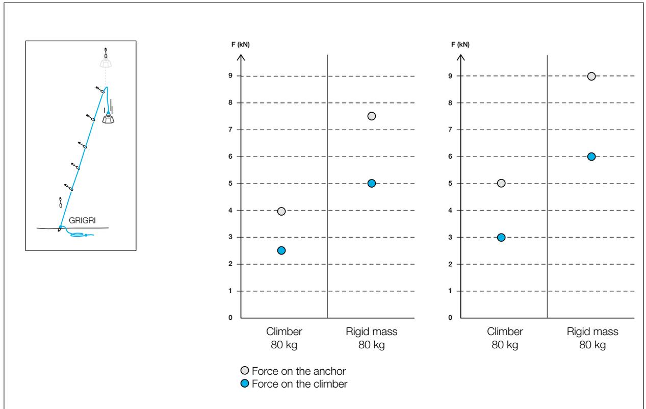
These tests revealed very significant differences between the two protocols: the force on the climber increases by up to 70% with a rigid mass.
