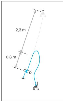
The dynamic test in the EN 892 standard consists of dropping a metal mass guided by two vertical rails. All dynamic ropes are subjected to this test.
