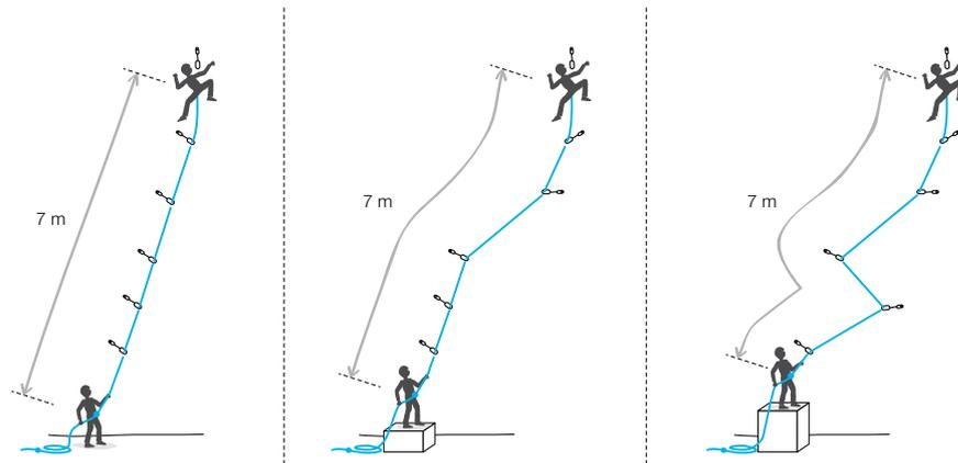
Only the drag was changed, the other parameters were constant. The belayer was gradually raised to keep the same rope length regardless of the rope path.
