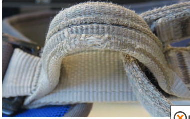
• Worn tie-in point
