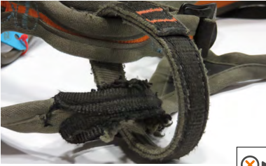
• Worn tie-in point
